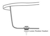
6. Take the drain tee and attach it to the strainer from underneath the bathtub. Tighten as much as possible.
