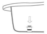
5. Take the drain tee and unscrew the right-handed side cap to connect to the overflow. There will be one gasket that you will remove to use to attach to the overflow drain. Set it aside for now.
