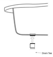
6. Insert the drain ell into the drain tee and screw in tightly. The use of threaded plumbing tape may be necessary at the joint to prevent leakage. This can be done at your discretion.
