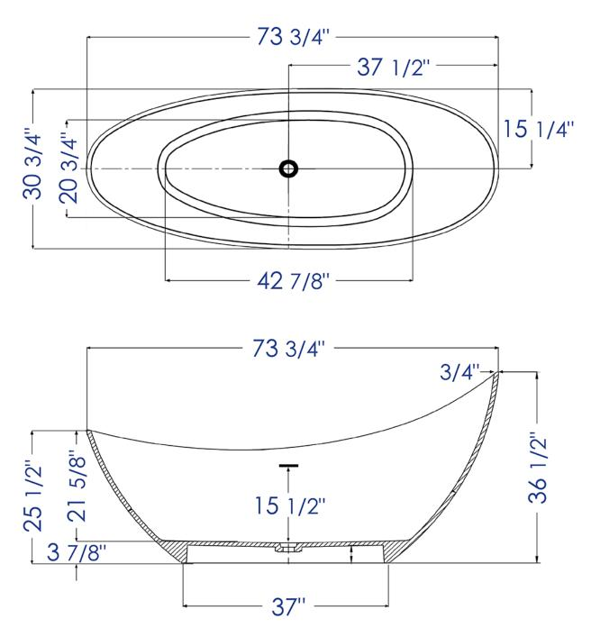
Please Note; Due to thermal expansion and contraction, the total dimension of the tub will have +-2% error, these dimensions are for reference only.
