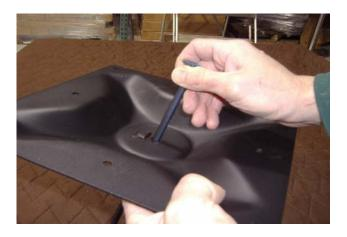
**4**- Put the end of the long threaded bolt into the hole of the alignment washer. Once this is done, align the 2 tabs of the alignment washer with the 2 slots in the column
