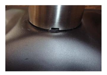
**6**- Inspect to see that all of the tabs are securely in their slots. Use the supplied tool to firmly tighten the nut. If the tabs did not initially slip into the slots, lightly tighten the nut enough allow some movement so the tabs and the slots can be properly lined up. When they are aligned, tighten the nut some more and lightly giggle the column or the mounting plate. The tabs should pop in the slots. Now tighten firmly
