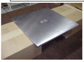
2- To protect the stainless surface against scratches the protective film can be left on the base plate until the assembly is complete. If the base plate did not come with the protective film, strips of masking tape can be placed over the alignment washer to protect the stainless surfaces against scratches. Note: The masking tape is not necessary if caution is taken to not scratch the stainless surface
