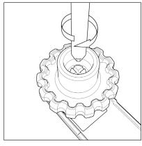
Mount the assembled levelers to the base using a #3 Phillips screwdriver.
