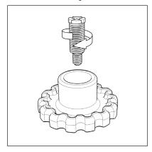
Thread the bolt into each leveler.
