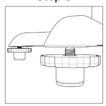
Adjust your table base by turning the PronToe until the base is level.
