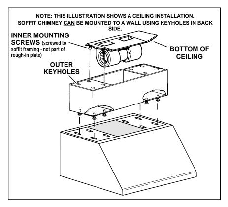
This Soffit Chimney takes the place of a soffit in vertically ducted or horizontally ducted installations.
