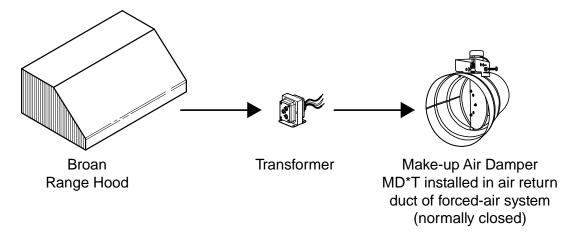
The Damper fully opens or closes based on a direct signal from a compatible BEST or Broan range hood which is "MD-capable." This signal is triggered by the operation of the range hood, which is sent through a hard wired connection between the two devices using a Broan-supplied transformer. Only those BEST, NuTone, or Broan range hoods which are MD-capable may be used for this application.
