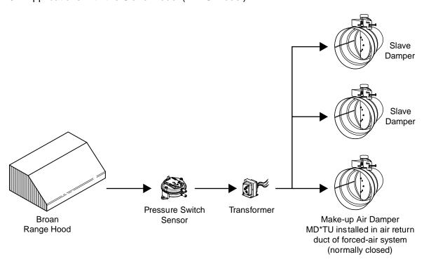
Any Other Model of Damper (LinkLogic<sup>™</sup>, Direct-Wired, or Universal)
