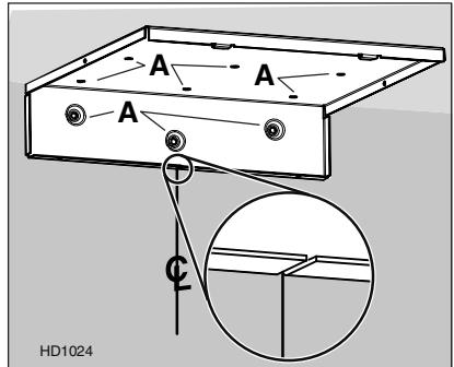
Using 4 no. 8 x 3/8" provided screws, assemble the 6" round adapter to the lower plenum plate.
