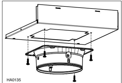
Assemble the lower plenum plate and 6" round adapter assembly to the upper plate by inserting both tabs of the top plenum plate to their corresponding slots in lower plenum plate. Secure the plenum assembly using 2 no. 8-18 x 3/8" screws (included).
