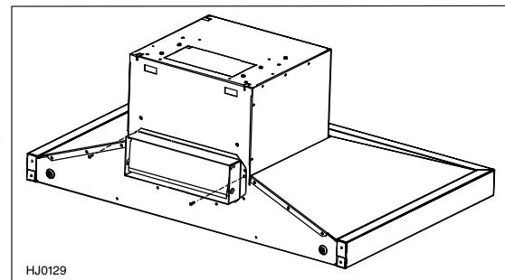
Secure the adapter/damper to the back of the hood using 2 no. 8 x 3/8" screws (included). Seal the adapter/damper to the hood using metal foil duct tape.
