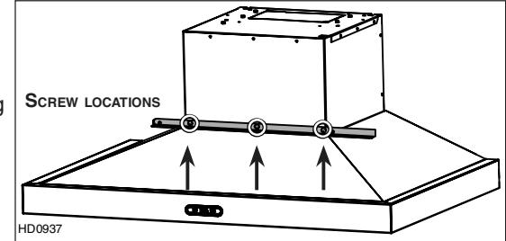
Before installation, remove and discard the shipping bracket (in grey) and its retaining screws. See illustration on the right.
