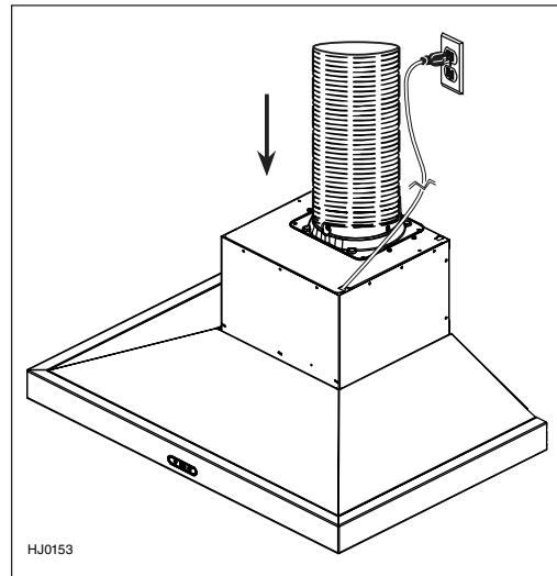
Stretch the flexible metal duct up to the plenum, over the adapter. Use metal foil duct tape to seal the joint.
