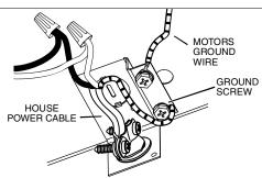
1] Connect House Power Cable to range hood wiring: BLACK to BLACK, WHITE to WHITE and GREEN or bare wire under GREEN ground screw.
