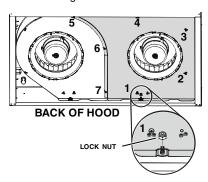
2 ] Reinstall the blower cover plate (shaded part on illustration above) using the lock nut and 7 screws previously removed in step 4 on page 10. Pay attention to screw 1 location; from back of hood point of view, it must be located on left side of the lock nut (see inset).
