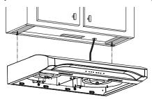
3] Secure the hood to the cabinet using two (2) no. 8 x 5/8" round head wood screws (included in parts bag). Insert one (1) screw per side, in the slots (as shown below). Attach power cable to the hood using the strain relief.
