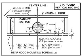
2] Install half-way two (2) ROUND HEAD no. 8 x 5/8" mounting screws into shims/cabinet, according to the proper diagram above, the other 2 ROUND HEAD no. 8 x 5/8" mounting screws will be used later. (Mounting screws are included in parts bag, but wood shims and shim mounting screws are not included.)
