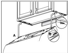
**4**] Unhook the rear holes from the brackets and hang the hood using its (2) recessed FRONT HOLES (**C** and **D**). **While holding the hood**, go to step **6**.
