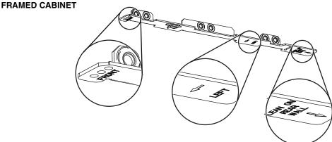
Refer to the marking on brackets to determine the correct installation side and orientation.
