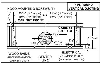
2] Install part-way four (4) ROUND HEAD no. 8 x 5/8" mounting screws into shims/cabinet, according to the proper diagram above. (Mounting screws are included in parts bag, but wood shims and shim mounting screws are not included).
