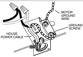
1] Connect House Power Cable to range hood wiring: BLACK to BLACK, WHITE to WHITE and GREEN or bare wire under GREEN ground screw.
