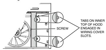
2 ] Reinstall wiring cover and attach it to the hood using its retaining screw.
