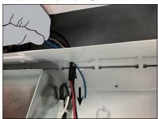
6 Close the electrical panel cover using 4 screws previously removed in step €.
