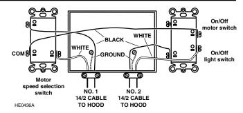
Install 2 included rocker switches at a convenient place for the user. Use two 14/2 cable to wire the switch box to the range hood (see diagram above).
