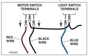
• Connect the RED wire disconnected from the motor switch to the RED wire from the kit, the BLACK wire disconnected from the motor switch to the ORANGE wire from the kit and the BLUE wire disconnected from the light switch to the BLUE wire from the kit. Route the wires to the wiring compartment area (through the hole along the BLACK and WHITE wires).
