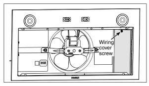
Disassemble the faceplate from the unit by removing its 4 retaining screws (two per side) Set aside the faceplate along with its screws.
