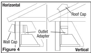
NOTE: For models using the B300, B500, and B600 blowers, a minimum of 6" diameter outlet adapter & ducting is required to achieve the proper air flow. The B900 requires a minimum of 8" diameter adapter and ducting. The B1125 requires a minimum 10" diameter adapter and ducting.
