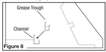
Install the baffle filters and any spacers included with the unit by inserting the top of the filter into the top channel of the hood, then slide the bottom of the filter into the bottom channel. The filters have a top and a bottom. The bottom of the filter will have small drain holes. These holes must be facing down towards the grease trough to be effective (Figure 9).
