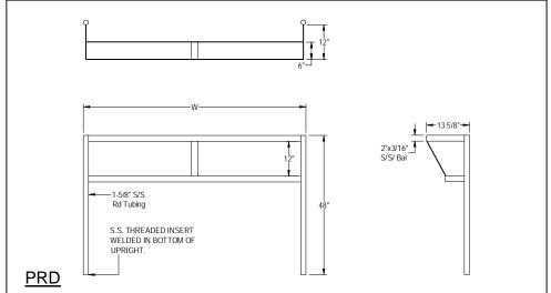
Shipped Welded set-Up
