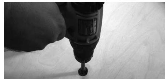
To prevent splintering, drill half way through on the back side and then the rest of the way through the front.
