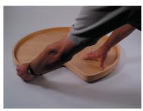
Step 4: Screw the SSusan down to the shelf (predrilling may be necessary) through the corner of the base plate. Repeat for the other 3 Corners.
