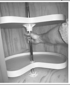
Turning a shelf upside down, position the Shelf Hub so that the positive stop indent is pointing to the left at 90 degrees from kidney cutout as pictured. Attach with four (4) - #6 x 1/2" Pan Head Phillips Wood Screws in the center of the mounting slots as shown. Turning shelf back over push the Shelf Collar into the top of the shelf until flush. Repeat with second shelf.
