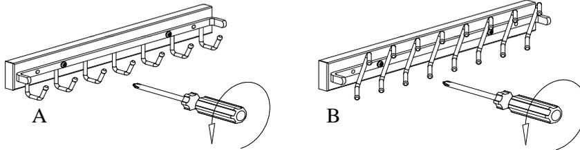
Step 2: Sliding out the housing and use 2 attached euro screws to fix slide on partition.
