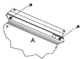
STEP 4. To relocate the valet, remove the rear screw on the valet rod, remove the plastic end cap, then pass it over the plastic bushing in the body.
