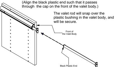
STEP 2. The valet body is mounted to the side of the closet using Euro Screws or #8 wood screw.
