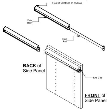
STEP 3. Once the valet body has been attached, slide the valet rod into the front of the valet body.
