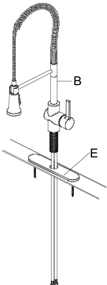
Insert the faucet assembly (B) through the hole in the escutcheon (E).
