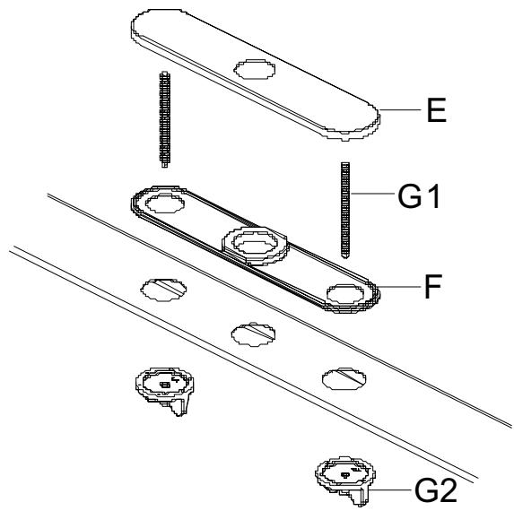
Before installation, remove the flange (D). Screw the bolts (G1) into the escutcheon (E) and ensure that the base plate (F) is pressed onto the escutcheon (E) before the escutcheon (E) is installed over the three holes in the sink. From underneath sink, hand tighten the mounting nuts (G2). Do not overtighten.
