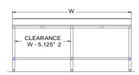
Shipped Standard Welded Set-Up
