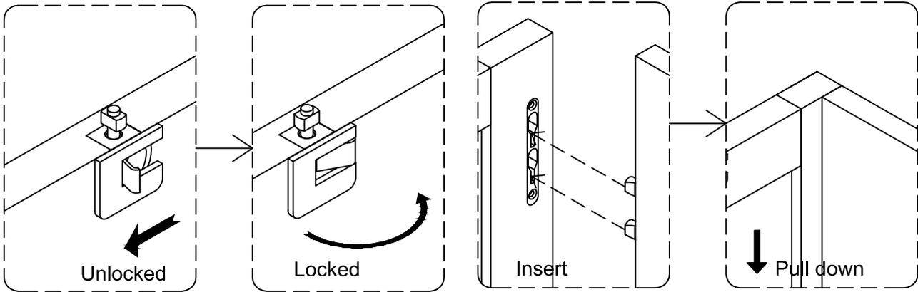
Reference the image above any time the instructions state "lock the hardware" or "insert hardware and pull down to lock".
