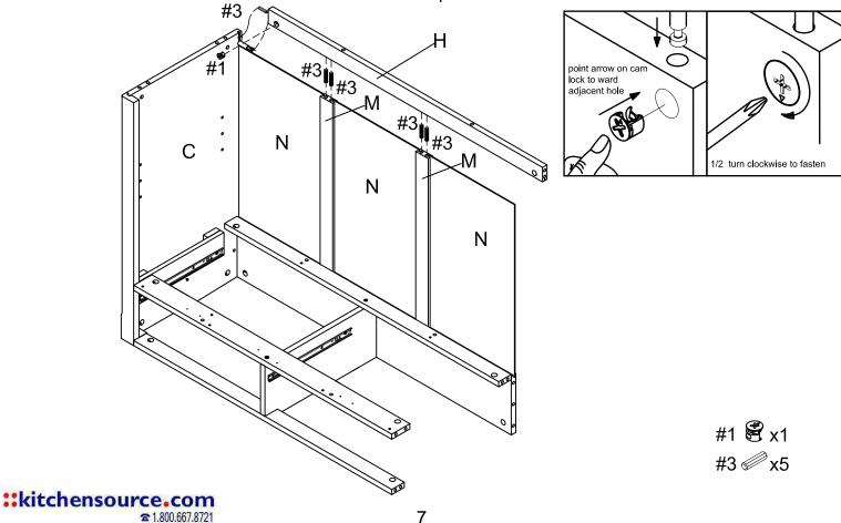
Step 7. Attach left panel (part B) to assembled unit (parts D, E, F, G, H & N) using wood dowels (part #3) and cam locks (part #1).
