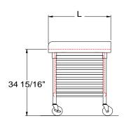
All units ship unassembled for reduced shipping cost. Units 7 ft. and larger are furnished with six legs. All dimensions are typical. Tolerance +/- .500".
