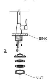
3. PLACE THE NEW FAUCET IN POSITION ON THE SINK. FROM UNDER THE SINK, PUT PLASTIC HOLDER, RUBBER RING, METAL RING AND THREADED NUT ONTO THE PIN. TIGHTEN THE NUT.
