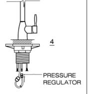
6. AFTER INSTALLATION IS COMPLETE, TURN ON THE WATER SUPPLY VALVES AND ALLOW BOTH HOT AND COLD WATER TO RUN AT LEAST ONE MINUTE EACH. WHILE WATER IS RUNNING, CHECK FOR LEAKS, ESPECIALLY AT HOOK-UPS TO SUPPLY LINES. TIGHTENING NUTS SLIGHTLY WILL STOP ANY MINOR LEAKS.
