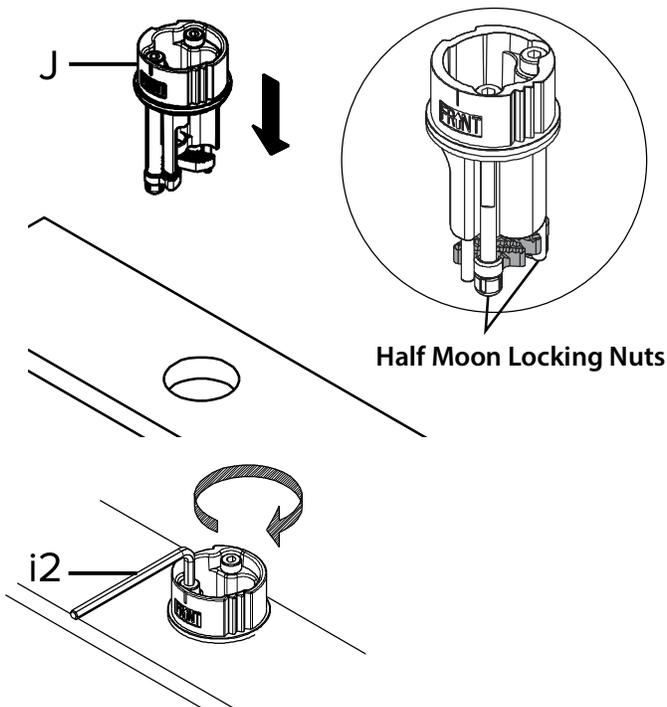
Insert base (J) into sink or countertop with "FR↑NT" facing forward. Tighten screws on base (J) with 4mm hex wrench (i2) until base is secure on sink or countertop
