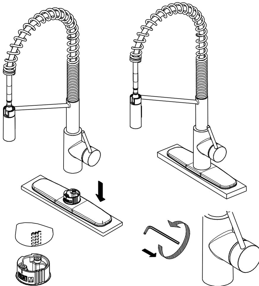
**Note:** "▲" on base should be in alignment with "▼" on faucet body.
