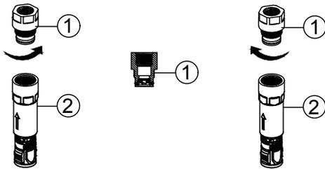
This faucet ships with a 1.8 GPM flow restrictor installed. An optional 2.2 GPM flow restrictor is also included in the box.
