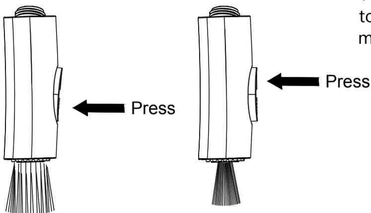
Turn faucet on. Press rocker switch to check if spray head (A) switches modes properly.
