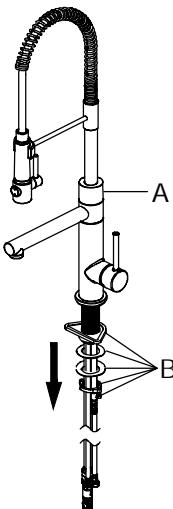
Shut off the water supply. Remove the old faucet. Clean the mounting surface. Remove the mounting hardware (B) from the faucet body (A).
