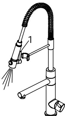
To activate the spray mode, simply press the handle (1) located under the spray head.
