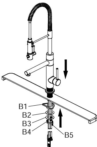
Insert the faucet through the hole in the sink or countertop. From underneath the sink, attach the seat (B1), rubber washer (B2), metal washer (B3), and nut (B4). Lock nut (B4) into position by tightening screws (B5).
