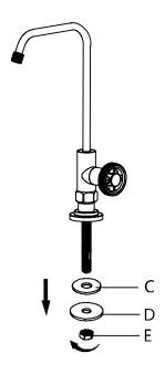
Remove the rubber washer (C), metal washer (D), and mounting nut (E) from the end of the stud.
