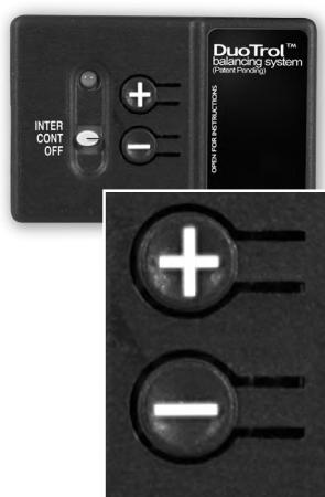
When the (+) button is pushed this will increase the CONT speed of both ventilation system motors from the previous settings.
