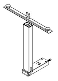
ASSEMBLE THE FOOT TO THE COLUMN
