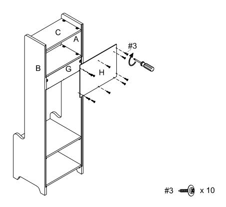
Step 7. Attach bottom back panel (part I) to assembled unit (parts A, B, F & G) using long screws (part #3) and phillips head screwdriver.
