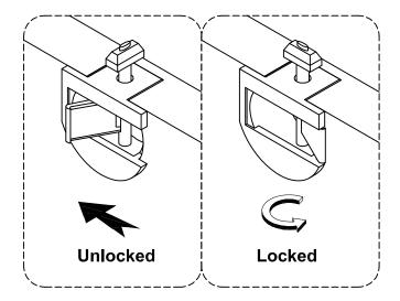
Reference the images above any time the instructions state "lock the hardware". Note: Be sure to check all hardware is locked when completed.
