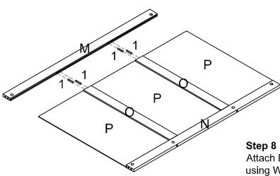
1 > x4 Attach Back Top Rail (M) to Rails (O) using Wood Dowels (Part #1) as shown.
