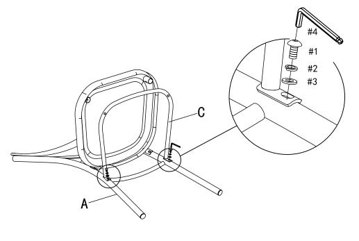
Step 3. Attach front legs (part D) to seat (part B) and stretcher (part C) using bolts (part #1), spring washers (part #2), flat washers (part #3) and allen wrench (part #4).
