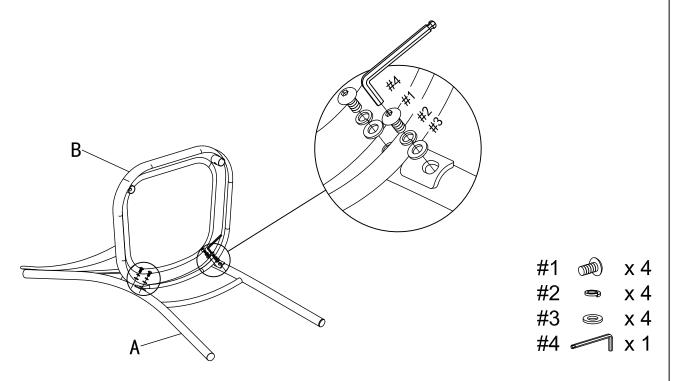
Step 2. Attach stretcher (part C) to back (part A) using bolts (part #1), spring washers (part #2), flat washers (part #3) and allen wrench (part #4).
