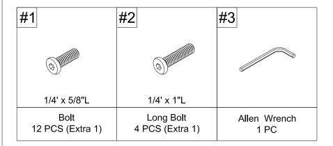
Step 1. Carefully lay marble top (part A) upside down on a flat, soft surface, such as carpet. Attach legs (part B) to marble top (part A) using bolts (part #1) and allen wrench (part #3).
