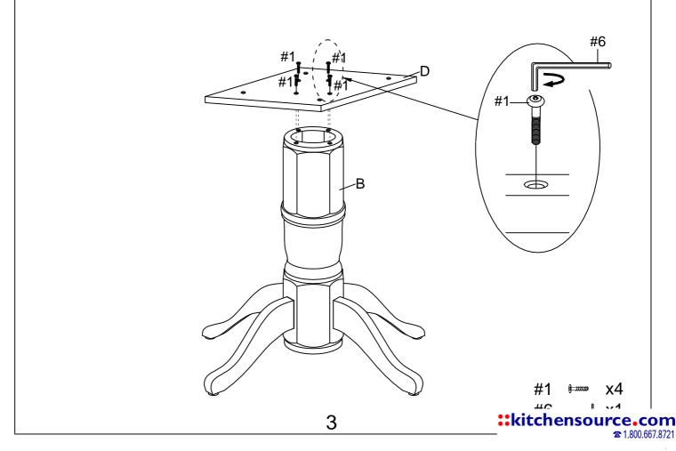
Step 3 . Carefully lay top (part A) upside down on a flat, soft surface, such as carpet. Attach assembled unit (parts B, C & D) to top (part A) using bolts (part #1), spring washers (part #2), flat washers (part #4) and allen wrench (part #6). Install adjustable levelers (part #5) to legs (part C).
