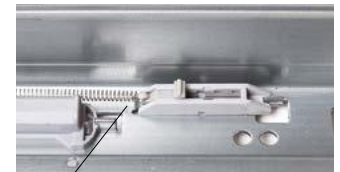
Adjust pull-force if needed to maintain smooth operation
