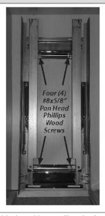
Place the slide base inside the cabinet, pulling the front cross member tight against the rear of the face frame. For frameless cabinets, set the front cross member back 3/4". For inset door applications, slide the base back from the above measurements plus the thickness of the door. Firmly secure with four (4) # 8 X 5/8" Pan Head Phillips Wood screws provided in the locations shown above. Replace the organizer onto the slide base. Proceed to the next step.
