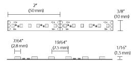
White Tunable FlexTape® can be used as a DIY option for flush and recessed Infinex. For other profiles, must be custom ordered.
