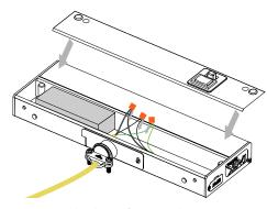
6. Fit wires back into fixture and snap cover shut. NOTE: Make sure the ground terminal ring remains aligned with the screw post when closing the fixture.
