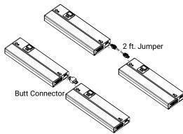
3. If connecting to another fixture, use either the butt connector or linking cable (sold separately). Connect the OUTPUT side of the connector to the OUTPUT side of the first fixture, then the INPUT side of the connector to the INPUT side of the second fixture. Repeat step 2 for mounting.
