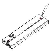
**2.** Remove the two screws on the top of the fixture. Gently pry open cover.
