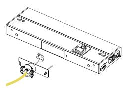
4. Feed input wire through the included cable connector, and then install the cable connector with wire run through it into the open knockout on the back door. Screw back door back to fixture.
