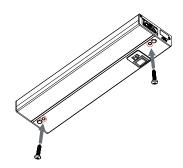
Place fixture in appropriate location and tighten mounting screws through holes on the fixture.
