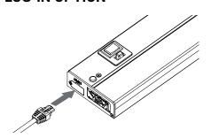
Plug power cord into the port on the end cap
