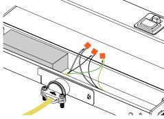
5. Strip wire 3/8" and connect the input power to the three push connectors inside the fixture. Black to black wire connector, white to white, and GROUND to the yellow-green wire connector.
