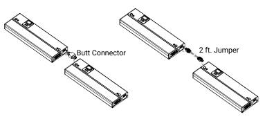
8. If connecting to another fixture, use either the butt connector or linking cable (sold separately). Connect the OUTPUT side of the connector to the OUTPUT side of the first fixture, then the INPUT side of the connector to the INPUT side of the second fixture. Repeat step 7 for mounting.
