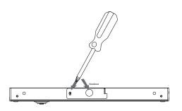
Punch out the knockout hole on the back door; unscrew round screw and remove the back door from the window by sliding it to the side.
