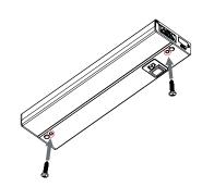
Place fixture in mounting location. Tighten mounting screws through holes on the fixture cover. Plug fixture into 120-volt power source. Plug mounting holes with provided caps to match fixture finish.
