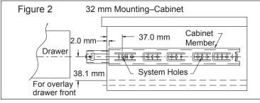
Use only the 32 mm system holes or the wood screw holes located at the tip of the breathing tabs. Do not use any other holes on the cabinet member for mounting (Figure 3).
