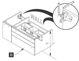
3 Apply a bid of silicone and hang the cabinet (D) on the brackets (E).
