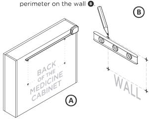
Once marked, drill the holes in the wall **G**. \*Insert the anchors in the holes **①**.
