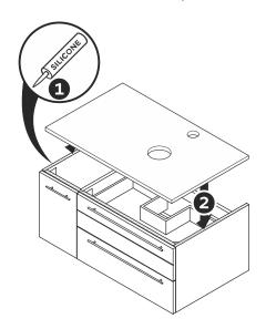
6 Apply a bead of silicone on top of a counter top and bottom of the sink. Connect sink to the counter top.
