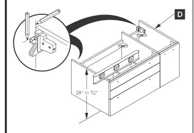
Apply a bid of the silicone and hang a cabinet (D) on the brackets (E).
