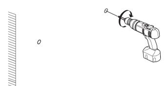
IMPORTANT: Consult an expert for the proper screws/bolts to use when attaching to various constructions, Screws provided do not attach to all wall constrution types. Anchors are not required if brackets are installed in stud.
