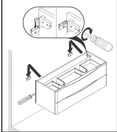
Apply a bead of silicone on the top of the cabinet and place sink on the cabinet
