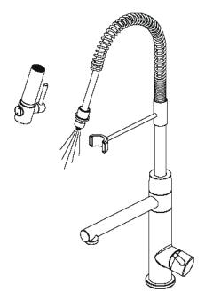
Pull the hose assembly out of the spout and remove the spray head by unscrewing it from the hose in a counterclockwise direction. Be sure to hold the end of the hose down into the sink and turn the faucet on to the warm position where it mixes hot and cold water.
