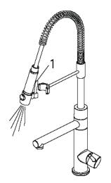
To activate the spray mode, simply press the handle (1) located under the spray head.
