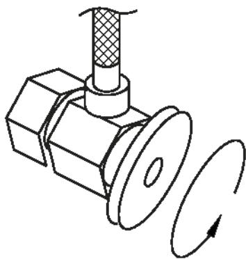
7. After installation is complete, remove the aerator. Turn on the water supply valves and allow both hot and cold water to run at least one minute each. While water is running, check for leaks, especially at hook-ups to supply lines. Tightening nuts slightly will stop any minor leaks.
