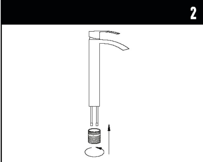
2. Connect flexible hoses to the brass pipes.
