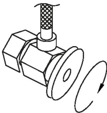
1. Shut off water supply. Remove old faucet and flexible hoses. Clean sink surface in preparation for the new faucet. Flush water connection at home to make sure no debris is stuck in the line.
