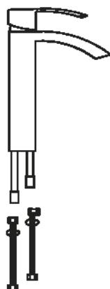
3. Connect flexible hoses to the brass pipes.
