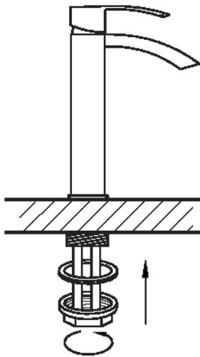
5. Place new faucet in the position on the sink. From under the sink, put rubber washer and thread nut onto the pin. Tighten nut.
