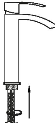
4. Place the metal base and rubber ring in to the slot at the bottom of the faucet.
