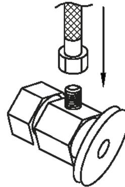
6. Connect female end of flexible hoses to the cold and hot water supply.
