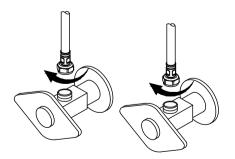
Attach waterlines to angle stops and tighten until snug. Turn on angle stops and check for leaks. (DO NOT TURN FAUCET ON)
