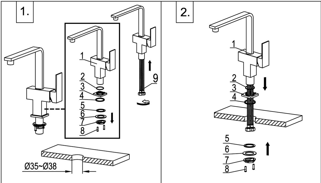
1.1) Drill a hole of Ø35~Ø38 on the installation deck. 2) Remove the nut (7), gasket(6) and washer C(5) from the main body. 3) Fix inlet pipes(9) onto the main body(1).
