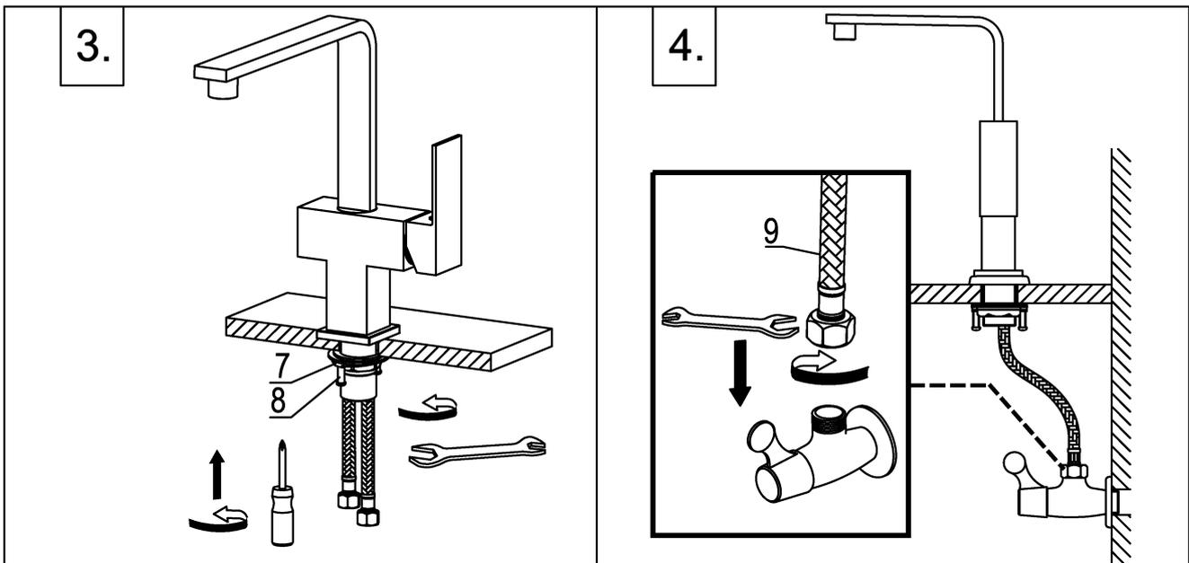
3. After adjusting to proper position of the faucet and base plate, fix the faucet by tightening nut (7) with a wrench and the two screws(8) with a Philips screwdriver.
