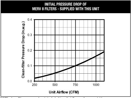
NOTE: clean filter pressure drop is included in unit airflow performance tables.
